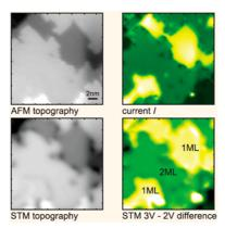
The researchers relied on scanning tunneling microscopy (STM) and conductive atomic force microscopy (AFM). Conductive AFM is itself a combination of STM and standard
